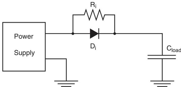
Diode  $D_i$  isolates the power supply from the load and in the event of a catastrophic failure in the power supply output section will prevent rapid discharge of the energy in  $C_{load}$  through the supply, which could present a safety hazard.  $D_i$  should have a reverse voltage rating at least 1.5 times the rating of the power supply, and a forward current rating at least 2 times the power supply capability.
