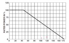
Derating (thermal resist.) LXP-150: 0.87 W/K (1.15 K/W)
