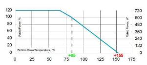
Derating (thermal resis.) UXC-600: 8.57 W/K (0.12K/W) Power rating: 600 W at 85°C bottom case temperature\*
