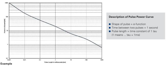
For the time-constant of 1 ms you can apply about 20 kW max., if the time between two such peaks is  $\geq$  1s
