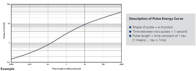
At 1 ms tau the LXP-20 with e.g. 1  $\Omega$  to 10  $\Omega$  can withstand an energy level of about 3 J, when the pulse pause time is  $\geq$  1s
