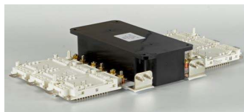
Fig. 1. Illustration of a single integrated cap / bus (SBE 700A243) sourcing two Infineon HybridPACK™ drive IGBT modules.
