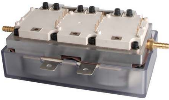
Fig. 4. Vertically integrated 100 kW inverter with improved topology and a measured ESL of 15 nH.
