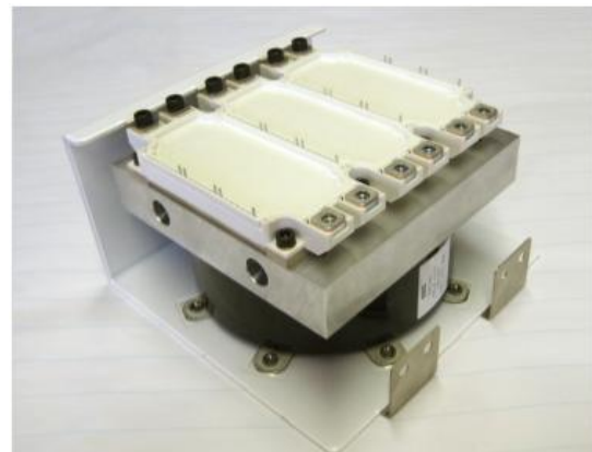
Fig. 3. Vertically integrated 100 kW inverter topology with an ESL of approximately 18.5 nH at the IGBT terminals.
