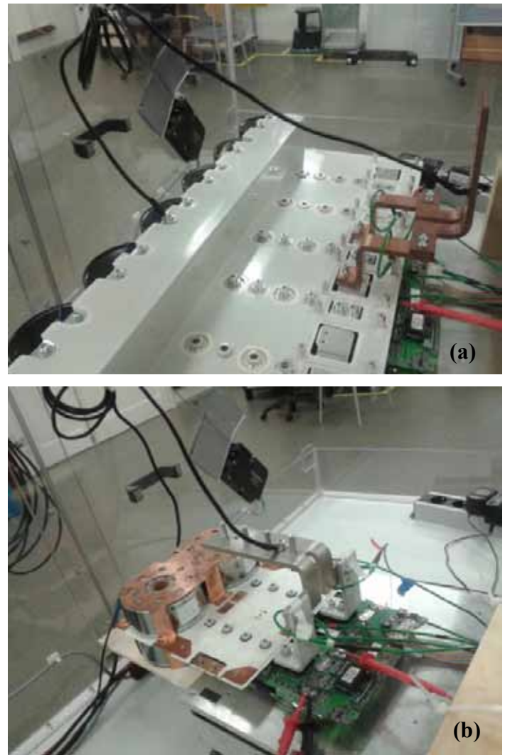
Figure 4: Bus bar with capacitors: (a) Danfoss, (b) SBE Power Ring Capacitors
