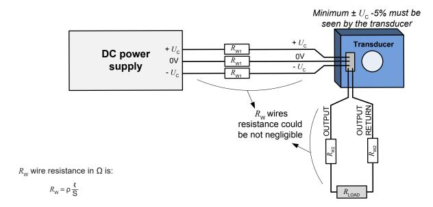
S: Cross section of wire in m<sup>2</sup>
